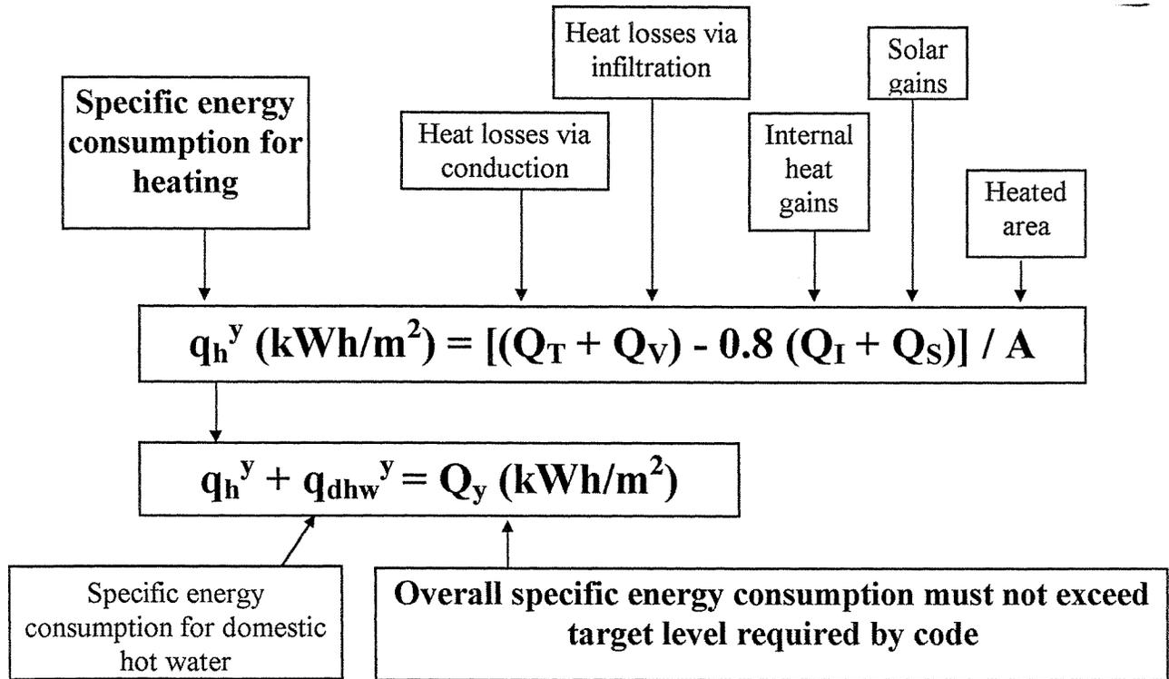
**Figure 1. Whole-Building Heat Balance and Performance-Based Compliance in Russian Regional Codes**
