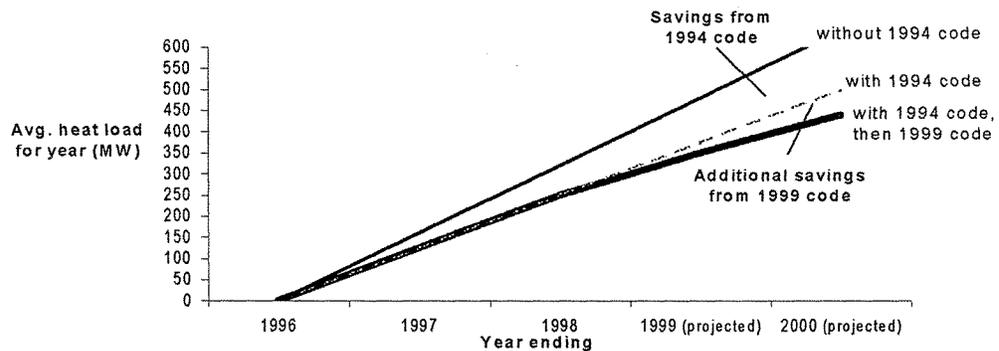
**Figure 3. Projected Heat-Load Savings from the 1994 and 1999 Moscow Building Energy Codes**
